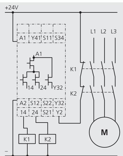
2-channel contactor control with feedback circuit monitoring
