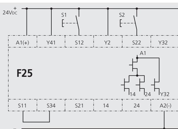
Two-hand switches connected directly to the supply voltage: +24V connected to terminal Y41 and S11 linked to S34
