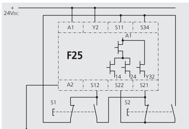
Two-hand switches connected to the dynamic outputs S11 and S21, S11 to be connected to S34
